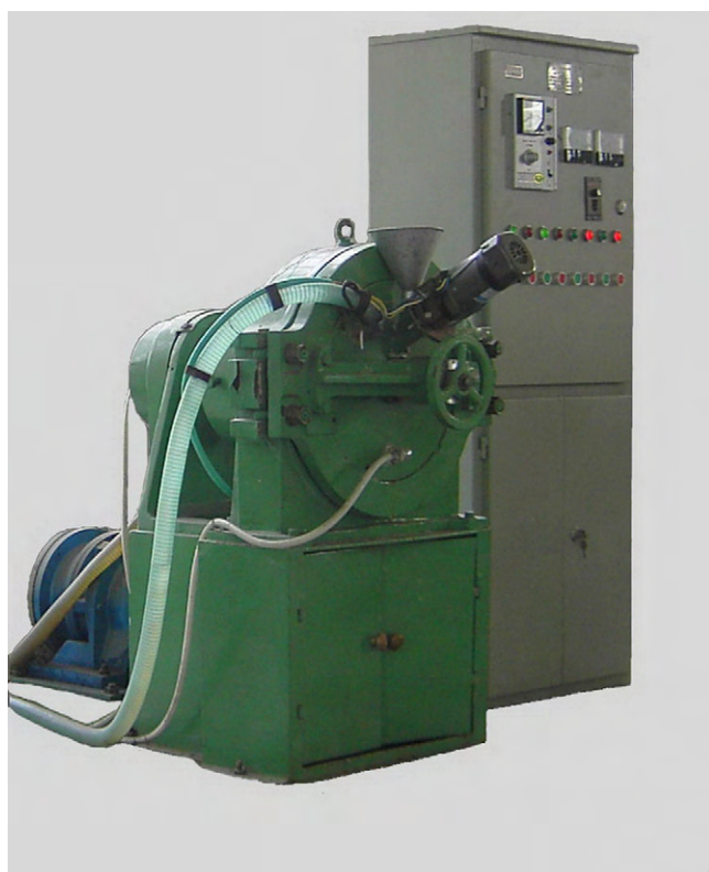
Fig. 1. Digital camera photograph of the pan-mill mechanochemical reactor.
